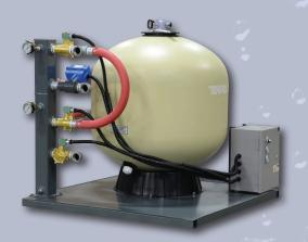
**PM SERIES SAND & GRAVEL FILTERS** have a media that removes free floating solids from plant circulating liquids that could cause blockages in manifolds and orifices in process equipment. Three sizes are offered so it can be configured to specific process requirements. Manual/automatic backflush and side stream pump options are available.
